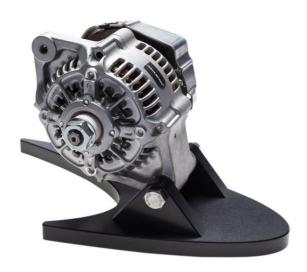
This alternator has a specially wound stator to achieve high power output in a small, low weight package. High current diodes are used in the rectifier and internal fans provide forced air cooling. The output is controlled by a regulator inside the alternator. The units are assembled with stiff brush springs and extra flexible wire to connect the stator to the rectifier.
