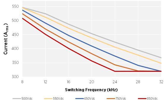
Peak Current vs Switching Frequency Map: 10s rating, 70°C Coolant @ 10L/min, Modulation Index = 1.0, Power Factor = 0.875
