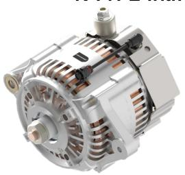
This alternator has a specially wound stator to achieve high power output in a small, low weight package. High current diodes are used in the rectifier and internal fans provide forced air cooling. The output is controlled by a regulator inside the alternator and is configurable over the CAN interface. The units are assembled with stiff brush springs and extra flexible wire to connect the stator to the rectifier.
